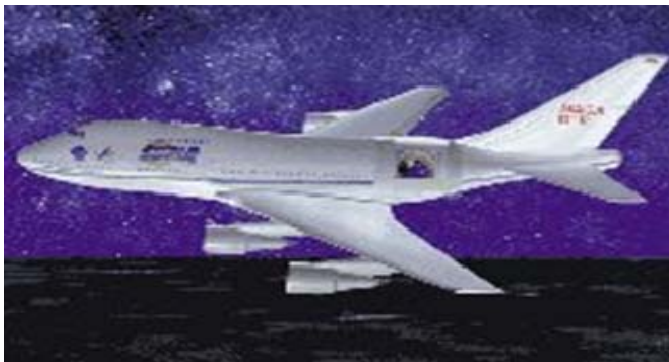
The aircraft has a 5 metre opening in its fuselage to house the telescope (Image: NASA)
