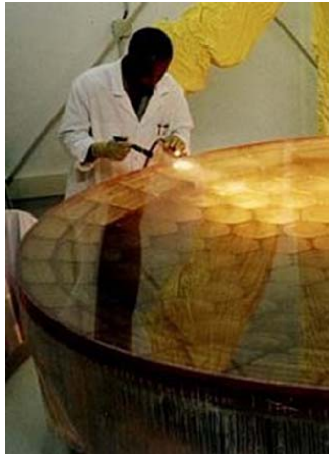
Polishing the telescope's 2.5 metre wide primary mirror (Image: DLR)
